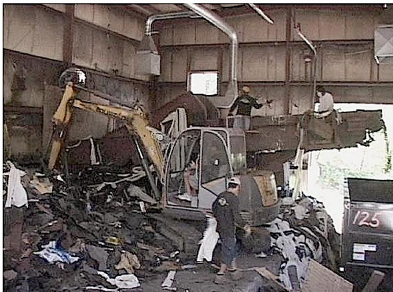
Trommel drum screens are often used to size material either before (see Picture 6) or after grinding (see Picture 14) depending on the system design and supply plan. Manual sorting to remove non-shingle debris is most often employed at the tipping floor in close coordination with the grapple crane or loader (see Picture 13).
