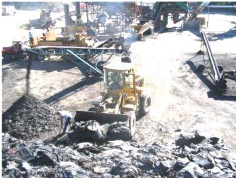
Other facilities relying on mixed waste sorting systems must employ more intensive front-end manual inspection and separation at the tear-off shingle recycling plant. Grapple cranes are often used instead of front end loaders to assist with pile management, rejecting large bulky items (e.g., scrap metal, plastic, wood), while also loading the cleaner tear-off shingle scrap into the feed hopper (see Pictures 6 and 13).
